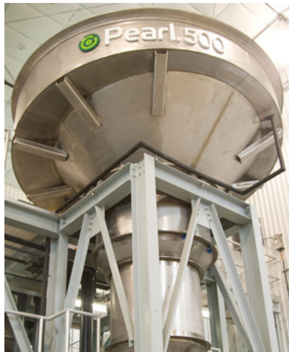
Ostara's Pearl Nutrient Recovery Process transforms municipal wastewater into Crystal Green.
